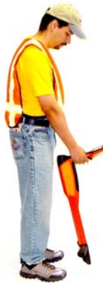
Figure 6-4: Receiver Position for Tracing
