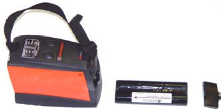
Figure 8-2: Replacing the D-Cell batteries with a NiMH battery pack
