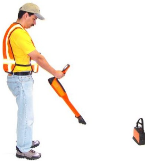
Figure 5-2: Aim Receiver at Transmitter
