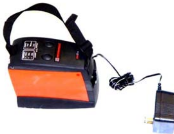
Figure 8-3: Recharging the NiMH Transmitter Battery with the Wall Mount Charger
