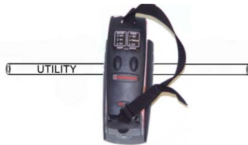
Figure 6-3: Transmitter Position for Inductive Tracing
