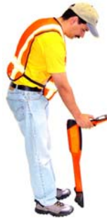
Figure 6-5: Receiver Position When Determining Depth
