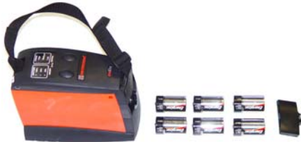
Figure 8-1: Replacing the D-Cell batteries
