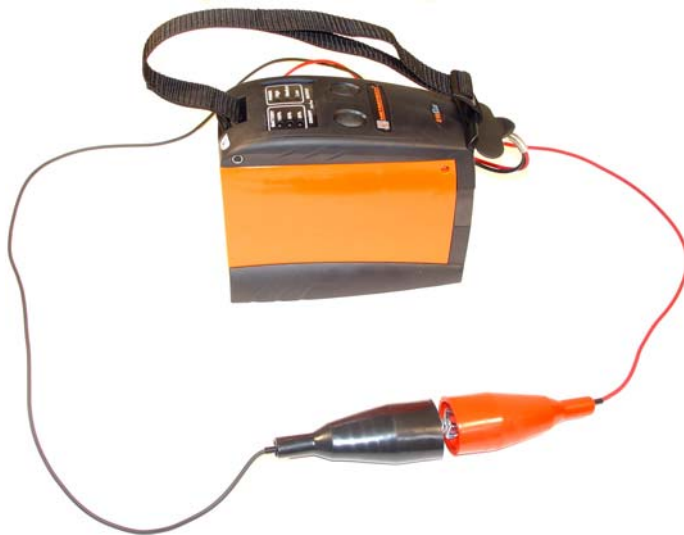
Figure 5-1: Connect Transmitter Leads
