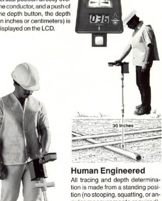
gular measurements required). Light in weight, the receiver is balanced for natural, comfortable right or left hand use, reducing operator fatigue. All instrument readouts are in line-of-sight. A single control switch activates all functions.
